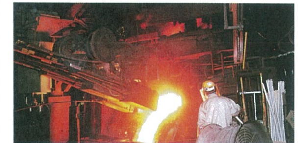
○Injecting oxygen gas into molten steel for melting and refining steel.
