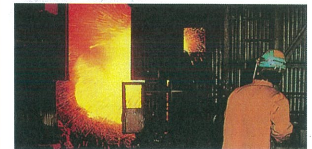
○Removing steel-slag mixture adhered inside oxygen converter by blowing oxygen gas.
